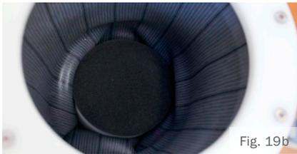
bearing cushion – with water „+ button“. To avoid membrane adhesion, lubricate the membrane above the distal bearing cushion with lubricating creme.
